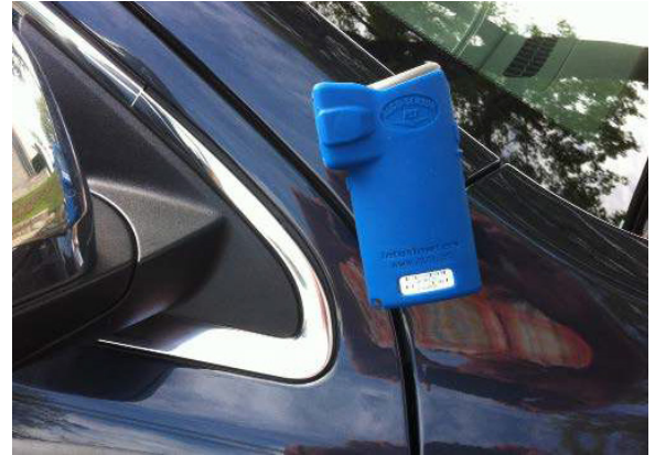
Bilateral magnets on outer sides of the instrument securely attach to ferrous metal surfaces.
